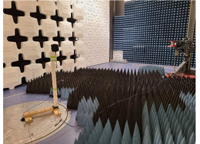
Fig. 2. Test setup used acquire the SVSWR data,
